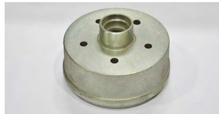
Bremstrommel Indespension 160 x 47 mm, Knott Typ, M12, 5 Loch LK: 112 mm
